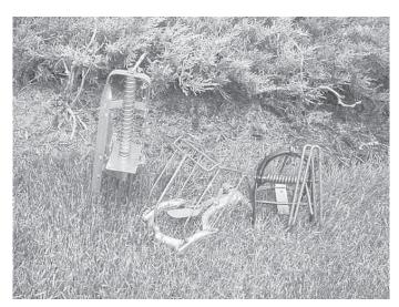
Pictured above are typical traps utilized in humane and effective mole control, including: harpoon, scissor-jaw, and choker loop style traps.
