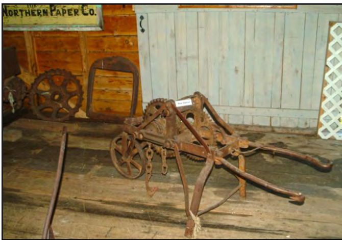
(Left) a Boom Tightener Displayed within the History Center at Churchill Depot
